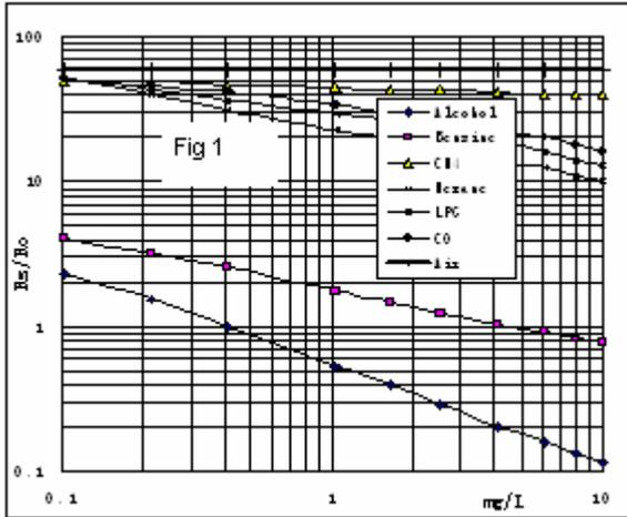
Fig.1 shows the typical sensitivity characteristics of the MQ-3, ordinate means resistance ratio of the sensor ( $R_s/R_o$ ), abscissa is concentration of gases.  $R_s$  means resistance in different gases,  $R_o$  means resistance of sensor in 0.4mg/l alcohol. All test are under standard test conditions.
