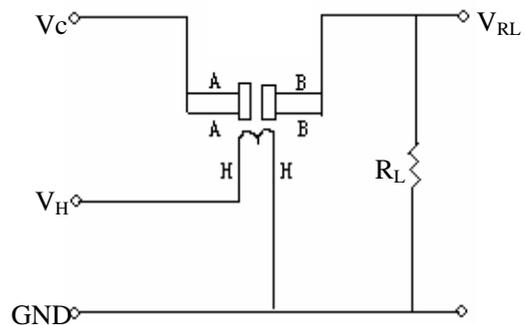
The above is basic test circuit of the sensor.
